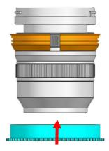
2. Insert the PL1635-F Focus gear on the plastic C-ring until it reaches the flange of the plastic C-ring.
