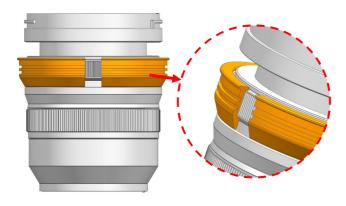
1. Insert the plastic C-ring as shown and place it over the lens
